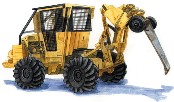
Figure 8.—A vibratory plow is sometimes used to disrupt grafted roots to prevent local spread of oak wilt.
